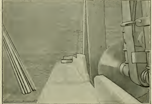
Swing Cut-off Saw for Car Sheathing.
